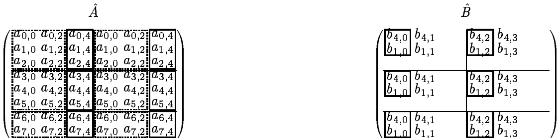
Figure 21c ( BB example): After processes (1,0) and (1,1) col broadcast matrix B , each process computes as much of the matrix multiplication as can be done locally (data in \hat{A} already used are marked with dashed boxes). Matrix A has used all of the data and will be broadcast.
