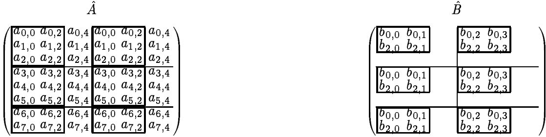
Figure 21b ( BB example): Matrix \hat{A} and matrix \hat{B} are temporary buffers storing the local matrices broadcast. Each process computes as much of the matrix multiplication as can be done locally (data in \hat{A} and \hat{B} used for matrix multiplication are marked with solid boxes). Matrix B has used all of the data and will be broadcast.
